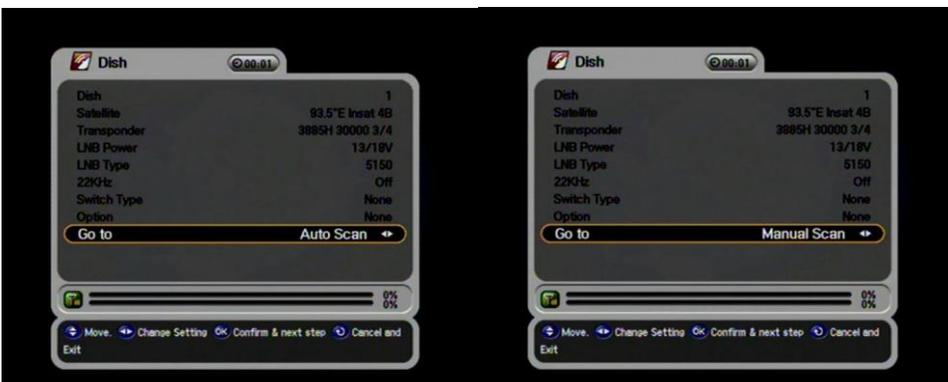
11) After Selecting manual Scan Option Please Check the signal Level and Signal Quality are more than 90.
