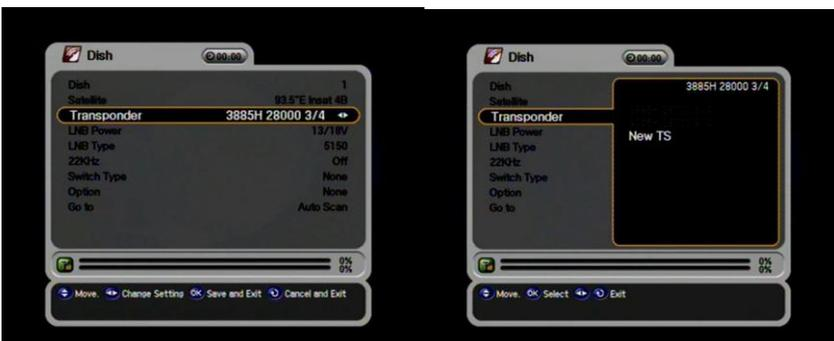
9) Input the frequency as 3885 and Symbol Rate and other Tuning Parameters as shown below.
